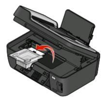
2 Raise the printer control panel, and then remove the ink cartridges from the paper exit tray.
