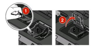
Remove the printhead from the disposable container.
