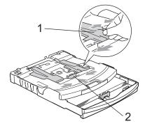
Put the photo paper into the photo bypass tray and gently adjust the paper side guides to the paper.
