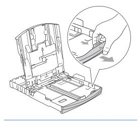
Gently adjust the paper side guides to the paper with both hands. Make sure the paper side guides touch the sides of the paper.
