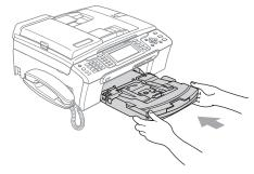
8 While holding the paper tray in place, pull out the paper support (1) until it clicks and unfold the paper support flap (2).
