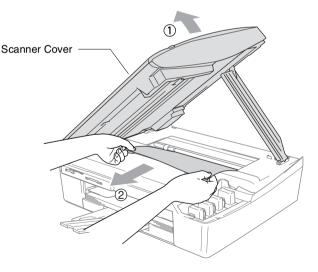
If the paper is jammed underneath the print head, disconnect the MFC from the power source so you can move the print head to take out the paper. **5** Lift the scanner cover to release the lock. Gently push the scanner cover support down and close the scanner cover.
