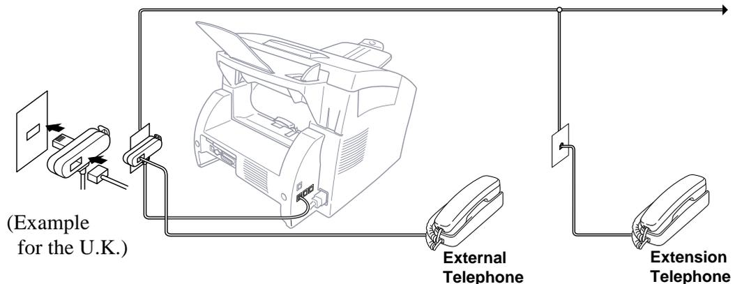
Whenever this external phone (or TAD) is in use, the screen displays **TELEPHONE**.
