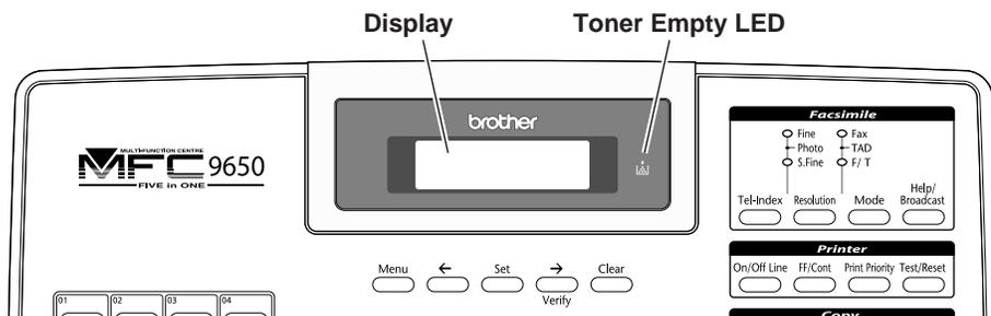
The Toner Empty LED light stays on and the display show **TONER EMPTY** to indicate that the toner is empty. Once this indication appears, your machine will not resume printing until you have installed a new toner cartridge.
