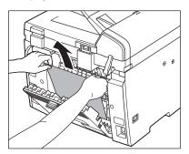
If the jammed paper is badly folded, similar to the folds of an accordion, ease the jammed paper loose and then pull it out from the machine.
