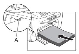
Adjust the paper guide rail to match the size of paper.
