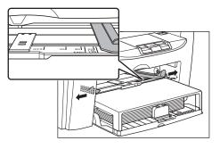
When setting paper, gently insert the paper into the multi-purpose tray with the print side up.
