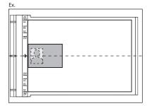
Align the center of a card with the arrow mark.
