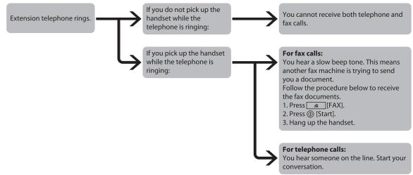
\*If <REMOTE RX> is set to <ON>, you can also start to receive fax documents by dialing from your telephone. (See "Receiving Documents Manually with an External Telephone (Remote RX)," on p. 5-39.)
