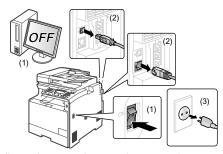
When installing and removing the optional accessories, be sure to turn the machine off, unplug the power plug, and then disconnect all the interface cables and power cord from the machine. Otherwise, the power cord or interface cables may be damaged, resulting in a fire or electrical shock.
