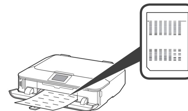
If an error message appears, tap OK, then proceed to ④. After installation is complete, refer to the **On-screen Manual** to redo Print Head Alignment.
