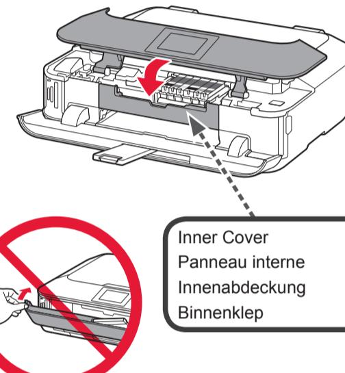
6 Check that the Inner Cover is closed, then close the Operation Panel.
