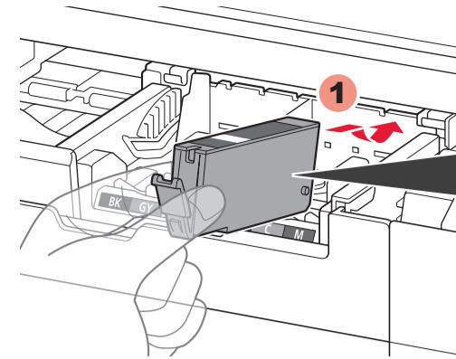
4 Insert and push down the ink tank into the matching color slot.
