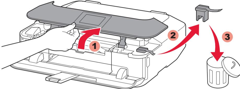
2 Open the Operation Panel. Remove the orange tape and protective material.
