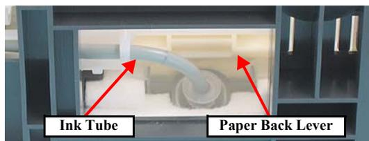
Figure 4-41. Paper Back Lever behind Ink Tube
