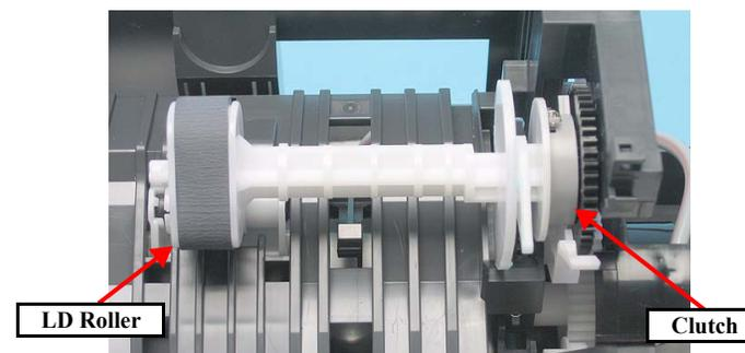
Figure 4-70. Assembling LD Roller (2)
