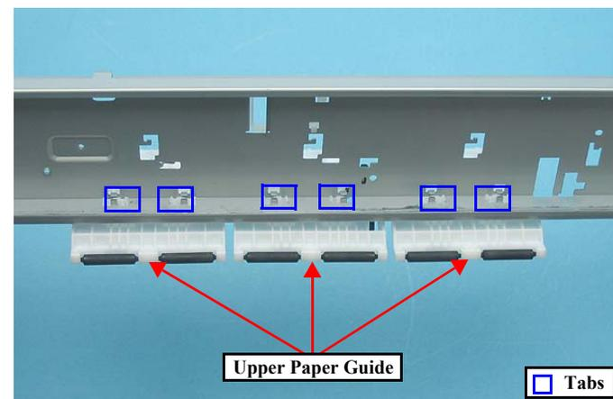
Figure 4-61. Removing Upper Paper Guide
