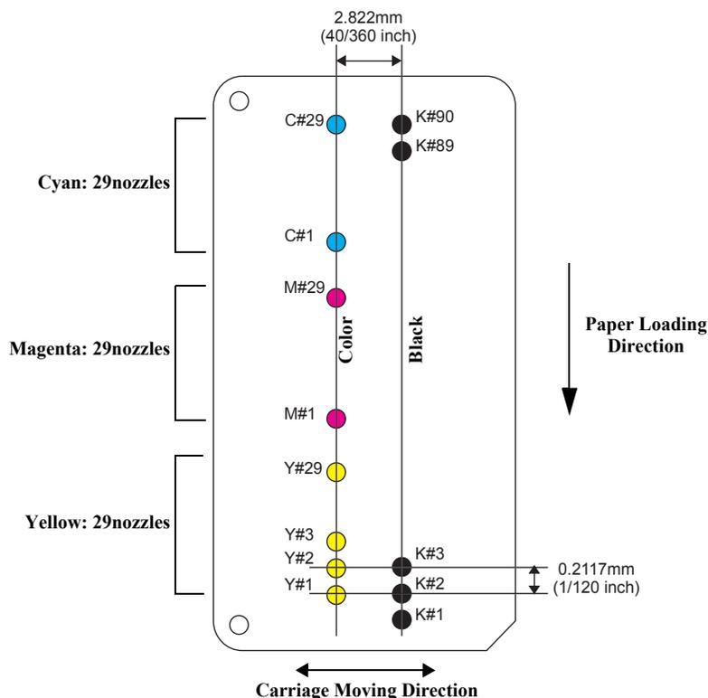
Figure 2-2. Nozzle Rear View
