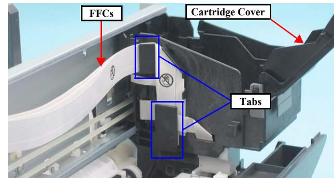
Figure 4-15. Releasing FFCs
