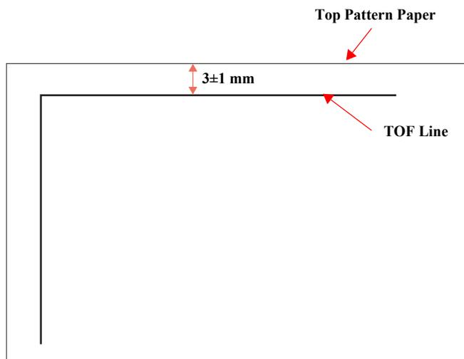
Figure 5-3. Top Margin adjustment Pattern Printing
