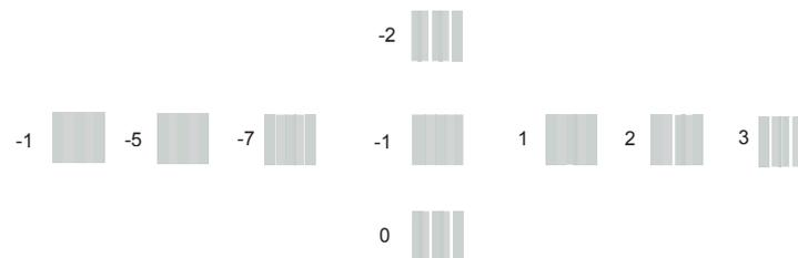
Figure 5-4. Bi-D adjustment Pattern Printing
