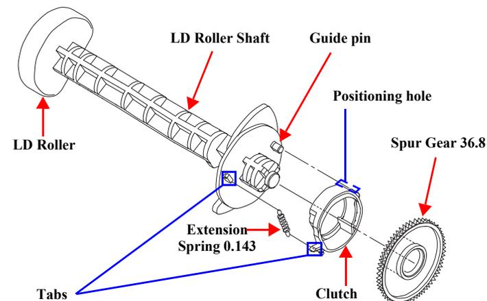
Figure 4-69. Assembling LD Roller (1)
