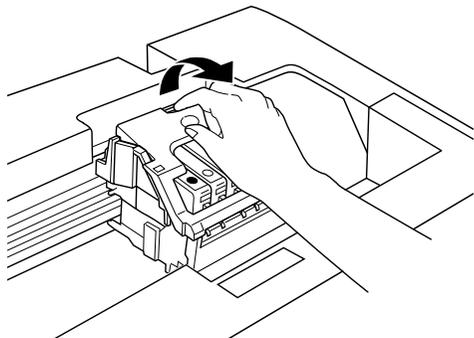
4. Remove the cartridge you need to replace. Press in the tab at the back of the cartridge to release it, then lift the cartridge straight out. Dispose of it carefully.
