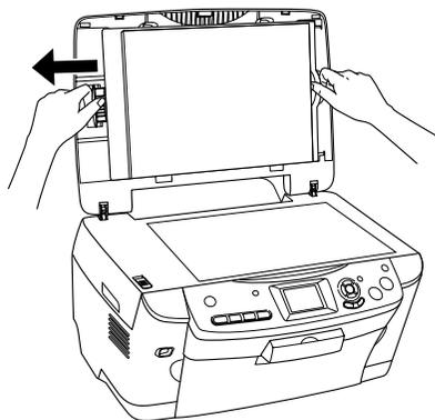
2. Remove the film holder from its storage place. (Remember to replace the film holder when you're done using it.)
