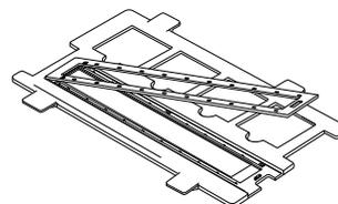
2. Slide your film strip into the holder with the duller (emulsion) side facing up. The top of the images should be facing the outside edge of the film holder and the images should be reversed.
