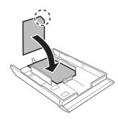
Load envelopes short edge first with the flap facing up and to the left. Next, check that the envelopes are not sticking out from the end of the cassette.
