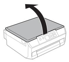
Place your original face-down on the scanner glass, and slide it to the front-right corner.
