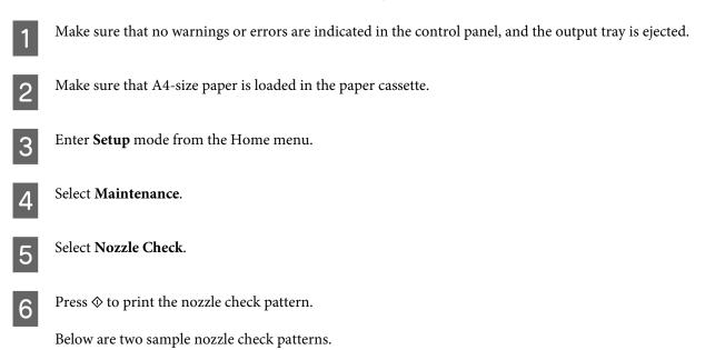
Compare the quality of the printed check page with the sample shown below. If there are no print quality problems, such as gaps or missing segments in the test lines, the print head is fine.
