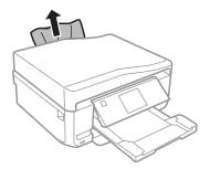
Open the scanner unit. Then remove all of the paper inside, including any torn pieces.
