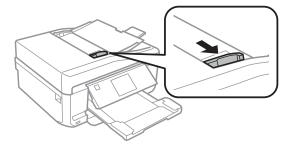
Insert the originals face-up and short edge first into the Automatic Document Feeder, and then slide the edge guide until it is flush with the originals.
