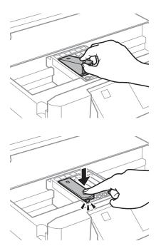
Put the cap back on to the removed cartridge's ink supply port. Dispose of the used cartridge properly.
