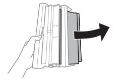
Open the rear cover and carefully remove the jammed paper.
