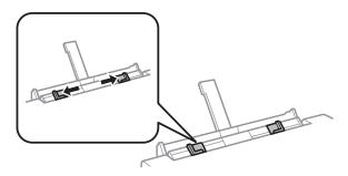
Load a single sheet of paper with the printable side face-up at the center of the rear paper feed slot, and then set the edge guide. The printable side is often whiter or brighter than the other side.
