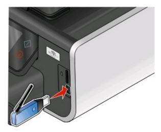
Bluetooth Dongle Connected appears on the display.
