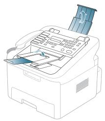
3. Load the original face down into the document feeder. Make sure that the bottom of the original stack matches the paper size marked on the document input tray.
