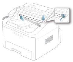
7. Reconnect the support and the control panel and then close the control panel firmly until it clicks into place.
