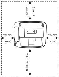
Printing is suitable for altitudes under 1,000 m (3,281 ft). Refer to the altitude setting to optimize your printing. Place the machine on a flat, stable surface so that there is no incline greater than 2 mm (0.08 inch). Otherwise, printing quality may be affected.
