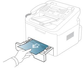
If the paper does not move when you pull, or if you do not see the paper in this area, check the fuser area around the toner cartridge (See "Inside the machine" on page 57).
