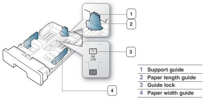
1. With one hand press and hold the guide lock, and with the other hand, hold the paper length guide and support guide together. Slide the paper length guide and support guide to locate them in the correct paper size slot.
