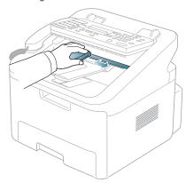
6. Replace the roller by inserting the left end first followed by the right end, then rotating the bushing until it locks into place.
