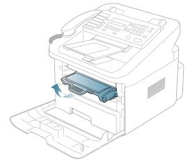
3. Thoroughly roll the cartridge five or six times to distribute the toner evenly inside the cartridge.
