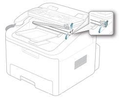
4. Wipe the roller surface with a soft cloth dampened with water.
